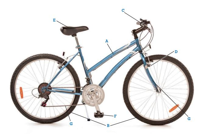
A. Frame B. Wheels C. Handlebars D. Brake
